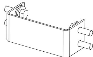
**Distribution Device Numbering Scheme Reversing Kit, P/N 565436 and 565437**
