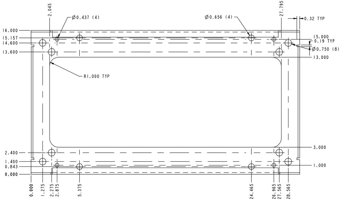
**List 03 and List 09 Floor Hole Drilling Pattern Dimensions**
