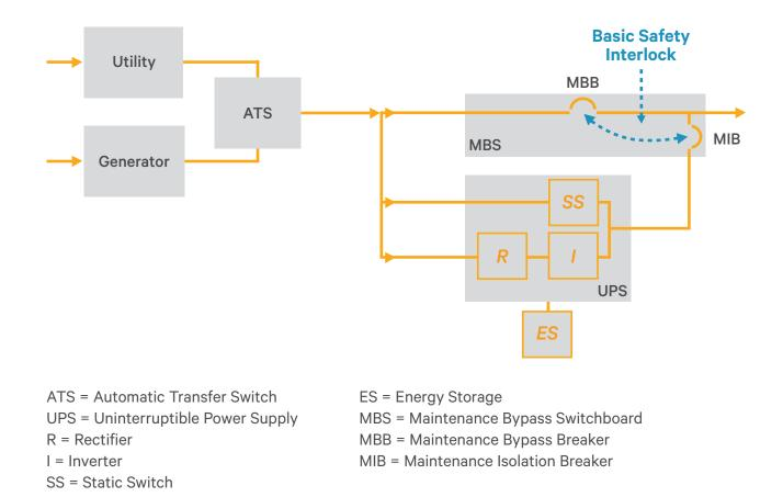
Figure 3: With the basic centralized configuration, the UPS is connected downstream from the Automatic Transfer Switch that transfers utility power between the utility and generator, and maintains power availability during this process. Diagram is for reference purposes only; not all inputs, breakers and TVSS products are shown.
