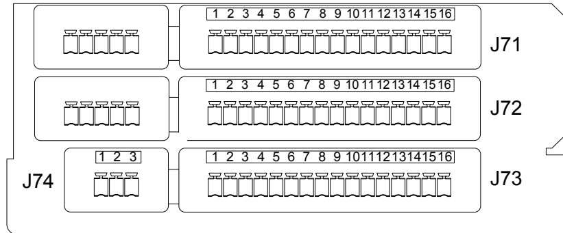
Figure 65 Control wiring, Programmable Relay Board
