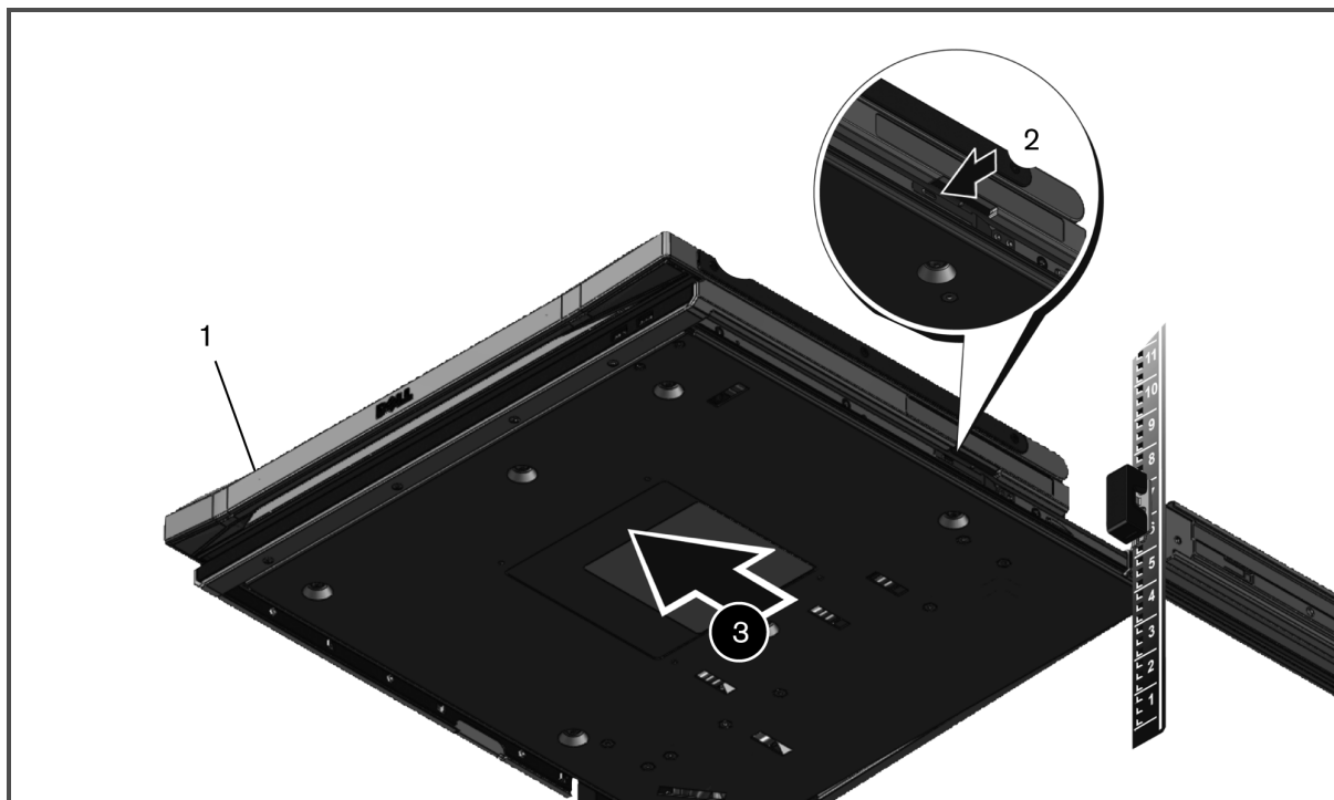
Figure 4.1 Removing the Console Tray From the Rack
