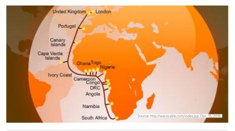
Capacity: 14.5T Bits/Sec; 4 Fiber pair
