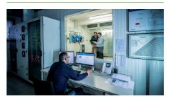
The Research & Development Validation Area n. 1 is specifically designed to test floor-mount units and can balance a thermal load of up to 150 kW with a chamber air temperature between 0°C and 60°C.
