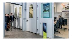
The Floor-Mount Validation Area meets the increasing requests for witness tests and specific product-type approvals. Equipped with a highly automated testing chamber, this validation area can balance a thermal load of up to 200 kW and can simulate a test environment within a temperature range of 0°C to 60°C.
