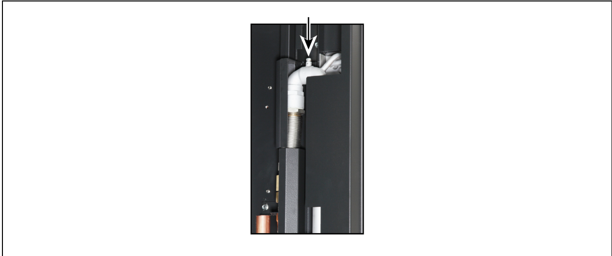
Figure 4.30 Schrader Valve to Bleed Air from Unit
