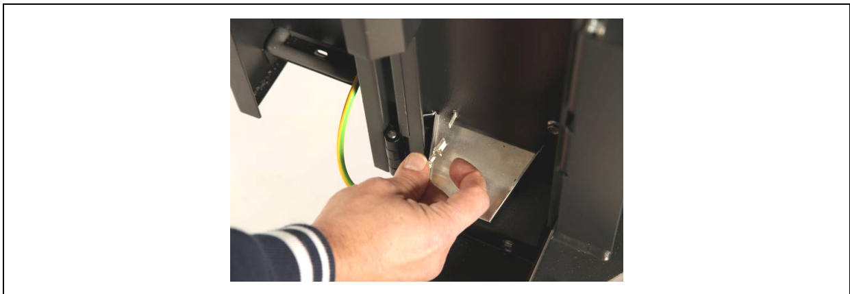
Figure 4.25 Attaching the Grounding Wire
