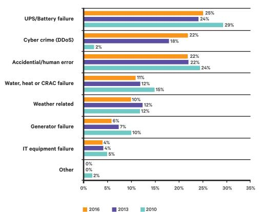
While batteries are one of the most "low-tech" components supporting today's mission-critical data centers, they are the most vulnerable part of an UPS system.
