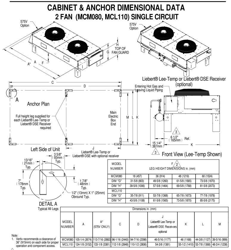
2. Cross bracing required for legs longer than 18" (457mm). Quantity varies per model & options selected.
