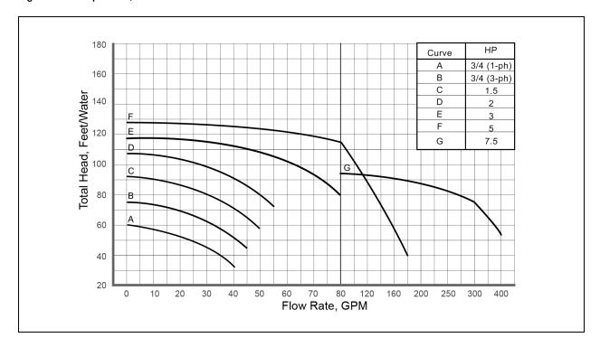
Figure 7.1 Pump Curve, 60 Hz
