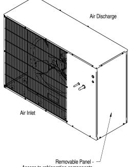
Access to refrigeration components, electrical components and connections
