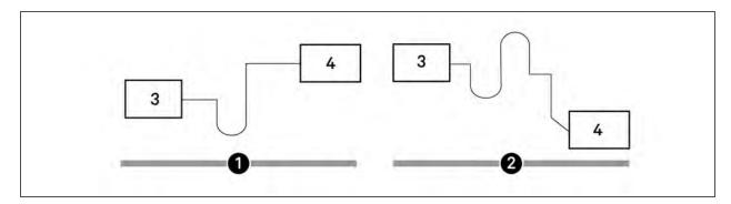
NOTE: Any horizontal pipe must be pitched down toward the condensing unit at a minimum rate of 1/2 in. (13 mm) per 10 ft. (3 m) to assure oil return to compressor.
