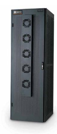
Each unit is rated for 1000 CFM (@60Hz). The unit mounts on the rear (inside or outside) of any standard rack (minimum 60" height). Two XDA units mounted side by side on the rear of a rack enclosure (2000 CFM capacity) move a nominal 14 KW heat load.
