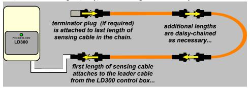
Some kits are supplied with a cable that is permanently terminated at one end; if your kit is one of these, then the terminated cable must be the last cable in the chain. If your kit does <u>not</u> include a pre-terminated cable, then the Terminator Plug must be attached to the last cable in the chain, as shown here.
