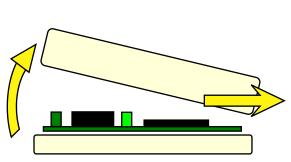
use hex key to remove the two setscrews in the bottom corners, then lift and push back the cover to remove it from the control box, as shown here.
