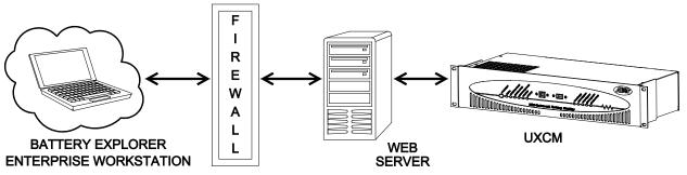
Figure 3 – Battery Xplorer Enterprise System Example using Ports 80 and 443 TCP
